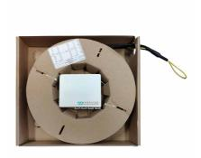
Plastic apartment optical termination box, pre-connected on both sides, with 4 SC/APC sockets and shooter; available with custom 81-89m of 4-fibre cable for FTTH multiservice installations; very useful solution to bring inside each individual housing unit all centralized services in the CSOE of FTTH installations.
